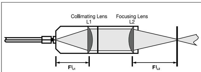
The first lens (collimator lens - L1) takes the rapidly diverging beam from the Fiber exit, and straightens, or collimates, it. This lens should be placed at a distance exactly equal to its focal length from the fiber exit face. If this is not done, the beam will not be collimated, and the imaging convention described below is void. The second lens (focusing lens - L2) acts as an objective, and focuses the beam to form an image of the fiber face.
